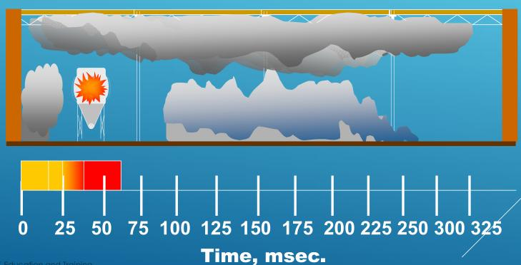
Primary deflagration breaks out of the equipment enclosure - creating a source of ignition
