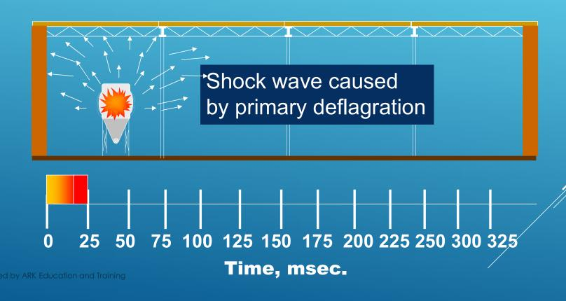
Shock waves reflected by surfaces within the building cause accumulated dust to go into suspension
